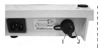
Connect the contact thermometer to the socket (I) on the rear panel of the instrument. Remove the jumper plug (J).
