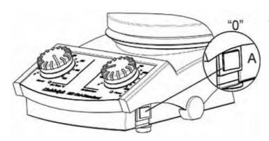
Before connecting the instrument to an AC power outlet, ensure that the rocker switch (A) is set to "0".
