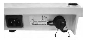
The *Hei-Con* and *Hei-Con-G* permit the temperature of the medium to be controlled in addition to that of the hotplate.
